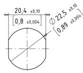
The SENSORswitch is secured against rotation by the illustrated hole. Metric and imperial measurements are used in drawings. Imperial measurements are marked with [].
